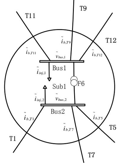
Fig 3. Topology for Substation 5 when all circuit breakers closed
