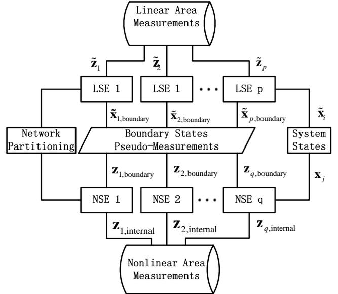
Fig 1. Flow chart of multi-area state estimation (LSE-Linear State Estimator, NSE-Nonlinear State Estimator)
