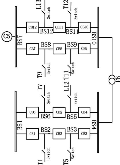
Fig 2. Circuit Breaker Oriented Model for Substation 5
