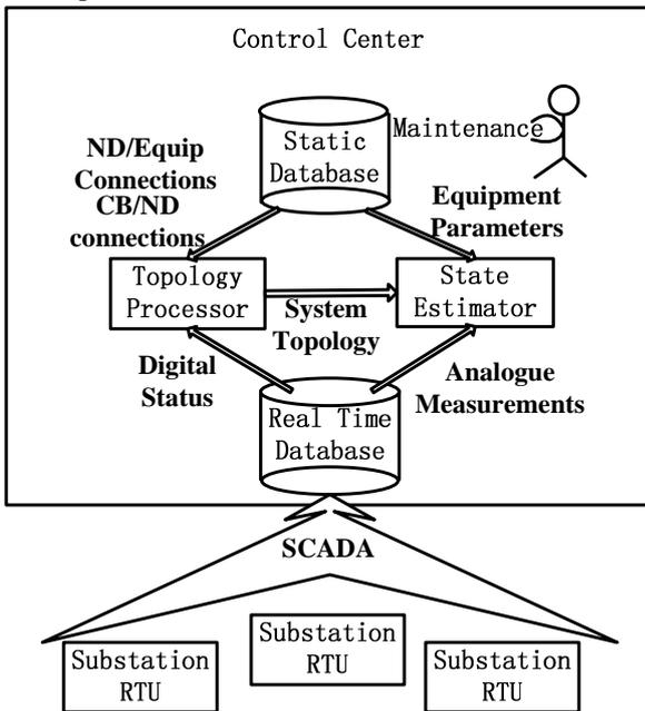
Fig 2. Traditional Real Time Modeling System and Database
