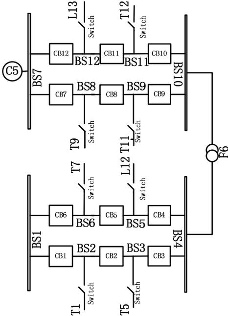
Fig 4. Circuit Breaker Oriented Substation Model
