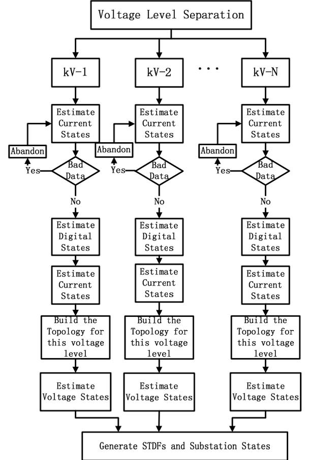
Fig 5. Flow Chart of the Substation Level State Estimator
