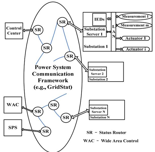
Fig 1. Power System Communication Infrastructure
