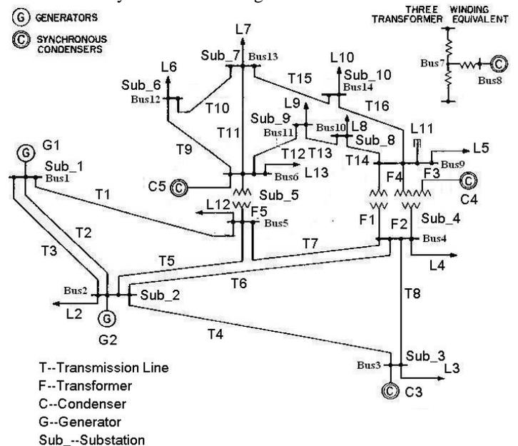
Fig 8. IEEE 14-bus system with named equipment
