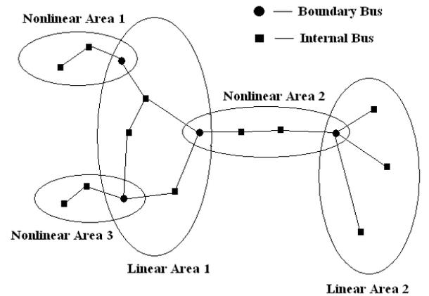
Fig 7. Multi-area network with boundary bus
